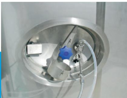
Easy access when needed: The inspection hatch offers a view into the tank interior. Optionally, the hatch can be equipped with a sampling device.
