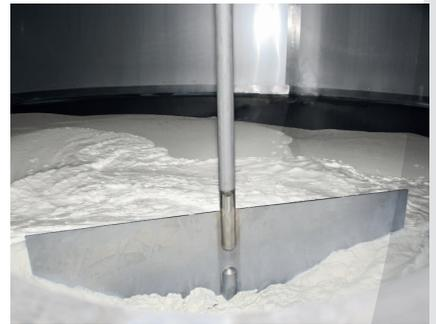
For perfect hygiene: Six high-performance nozzles ensure effective dynamics in the cleaning interval. Additionally, 4 separate in-line heating elements raise the water up to temperature in the main rinsing process. Minimum water consumption as well as economical metering of the cleaning agents are kept firmly under control by the ICool control system. In a final step the cone-shaped tank floor lets the milk and rinse water flow off quickly and completely.
