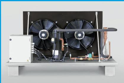
Designed to save energy: The scroll compressor and highly efficient condensers can be adjusted to the expected milk quantity. Altogether, 25 different cooling units with a refrigerating capacity between 3.82 and 30.7 kW/h and a milk cooling efficiency between 110 to 945 l/h are available.
