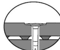
**i** tip: check to see if the fastening can be felt with a flat object made of metal (e.g. hammer) by sliding it over the fastening. If it can be felt, pound it in deeper!
