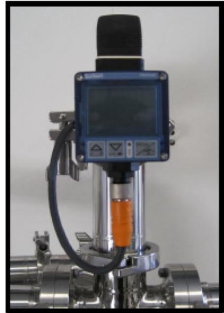
Our digital hygienic pressure gauge is fully adjustable enabling set up for individual milk delivery line specifications.
