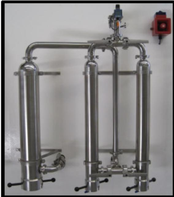
Twin 4" Milk Filter installed with our filter alert kit. Know when your Milk Filter is blocked before its too late.
