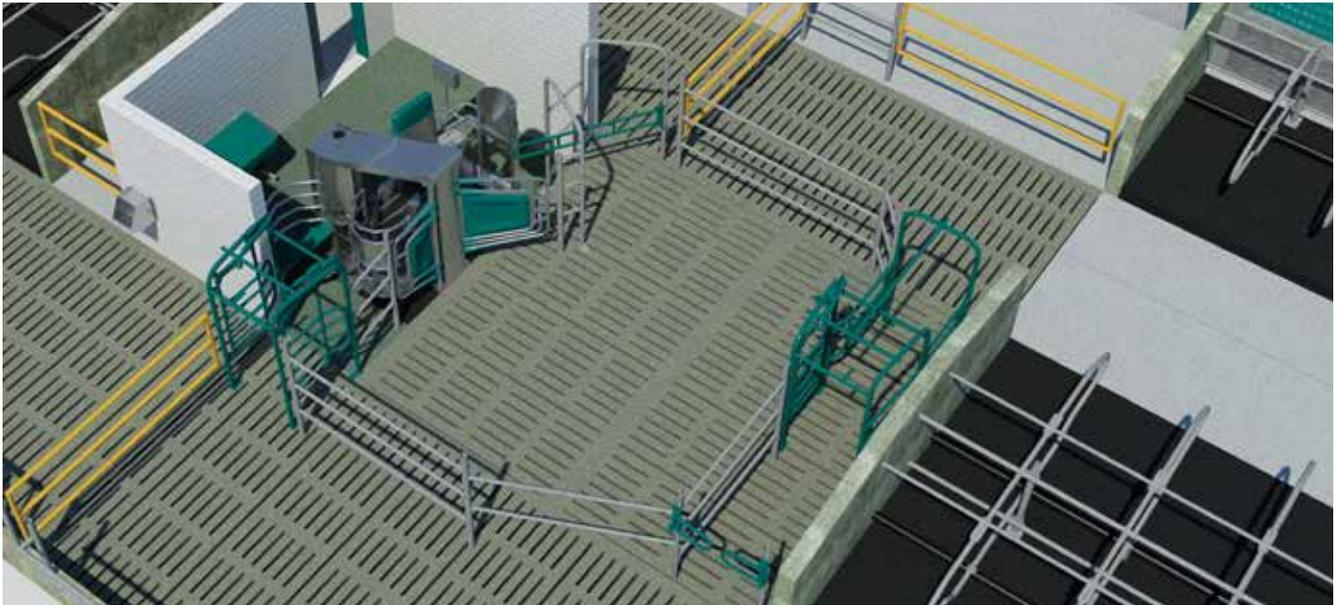
Selective guided cow traffic systems provide clear separation of the housing areas with the help of pre-selection, creating an optimal balance of feeding, resting and milking.
