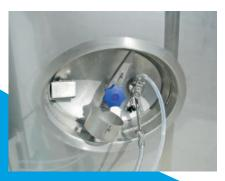
Easy access when needed: The inspection hatch offers a view into the tank interior. Optionally, the hatch can be equipped with a sampling device.
